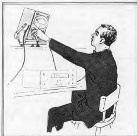
Figure 9. Various methods of placing the Flip-Tilt case for convenience in reading the meter.
