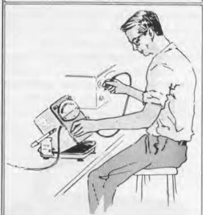
Figure 9. Various methods of placing the Flip-Tilt case for convenience in reading the meter.
