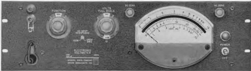
Figure 10. View of the Type 1806-AR Electronic Voltmeter for relay-rack mounting.
