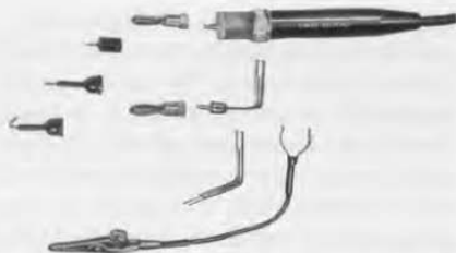
Figure 5. The ac probe and its accessory tips and ground clips.
